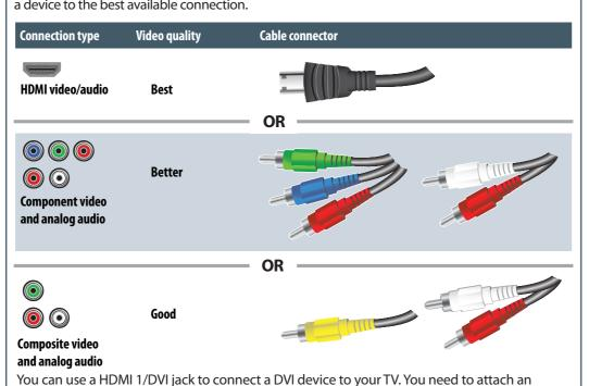
HDMI-to-DVI adapter to the end of the HDMI cable that connects to the DVI device's jack.
